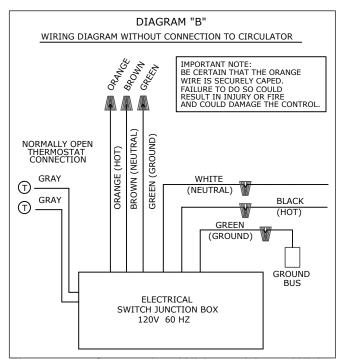
Figure 2-2: Connection Wiring without Wiring Central Heating Circulator
